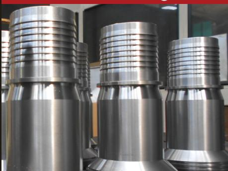
Precision CNC turning for components up to 400mm diameter and 1000mm length. Our advanced technology ensures high accuracy, tight tolerances, and superior surface finishes for every project.
