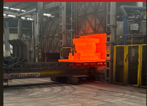
Featuring one of the UK's largest water quench systems alongside versatile polymer quench options. Our capabilities ensure precise control, improved material properties, and consistent results, meeting the highest standards for strength, durability, and performance.
